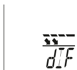
8. Differenza temperatura infrarossi (max. / min.)
